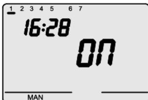
The manual operating mode activated by pressing the MODE key until the MAN message is displayed on the VDU.
