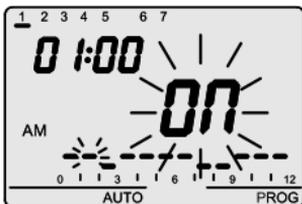
The message ON (or OFF) blinks on the VDU. The ▲▼ keys can be used to modify the output status. The modification takes effect starting from the time selected and extends until the next transition or until the end of the day that is being programmed if there are no subsequent transitions. The choice is confirmed by pressing the MODE key within 30 seconds.
