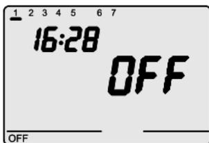
In **OFF** mode the N.A. relay contact is kept constantly open while the N.C. contact is closed.
